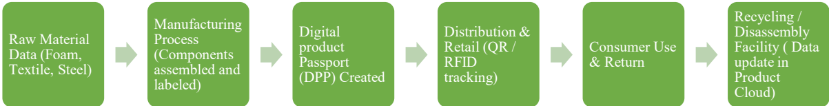
Figure 4: Digital product passport and traceability integration in mattress manufacturing (World Furniture Magazine, 2024)
